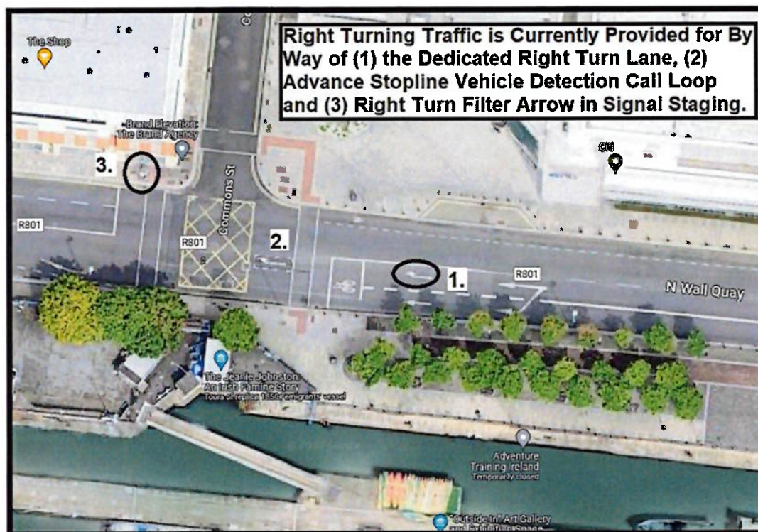
Figure 3.4: NRB Consulting Engineer’s Annotated Google Aerial Streetview of existing right turn lane.
